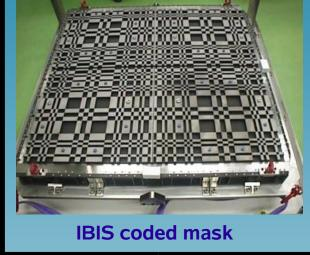
Opaque plates and holes optimally distributed. (Pattern of holes)
