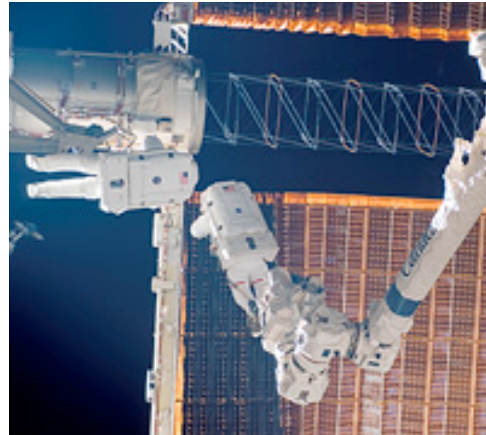
P6 solar array jam on ISS ESA/NASA, 2006
