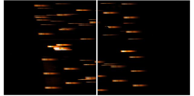
Exposure of an Argon lamp taken with the Prism during ground test. The MSA was configured in "slitlets" with sets of 4 alternating open/closed shutters. Spectra from four of the fixed slits can also be seen in the center/left, and the fifth slit in the center/right.
