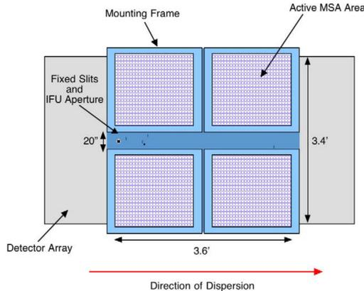
Schematic of NIRSpec apertures superimposed on the detector array FOV.
