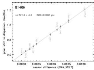
GWA position sensor voltage vs. spectral shift. Courtesy DeMarchi/ESA.
