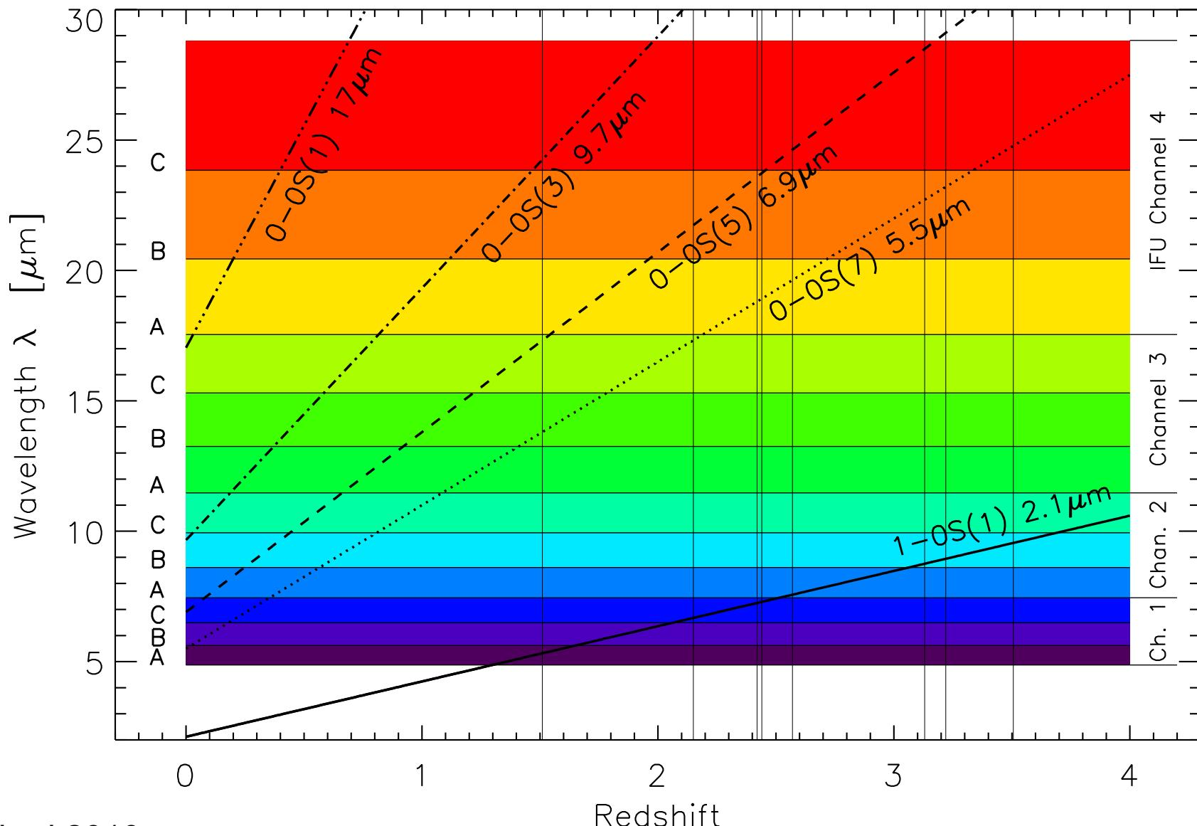
R=600-2400 spectroscopy, emission line, point source
