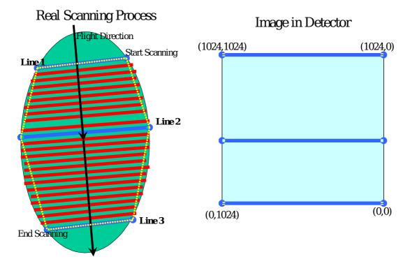
The description of the footprint will be completed by providing all of the instrumentrelated parameters for the "central point" of the each line. These parameters provide the necessary information to locate the footprint in the database. The figure above provides a visual representation of the schema.
