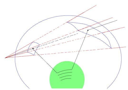
In this case, the center point of the line is defined as the projection on the body of the center point of the beam central line (black line in the figure).
