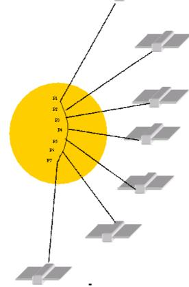
The figure shows how the footprint is created for an environment instrument.
