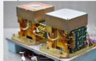
X-ray sensor and signal-processing electronics
