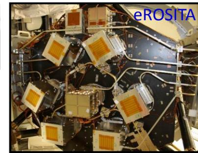
**Passive cooling** with heat pipes and radiators
