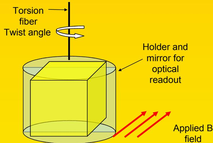
Measurement of *magnetic moment*:  $\vec{m}(t) = \vec{m}_0 + \frac{\chi V}{\mu_0} \vec{B}(t)$
