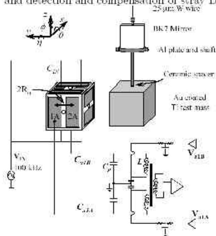
FIG. 1: Sensor electrode configuration and circuitry, with
