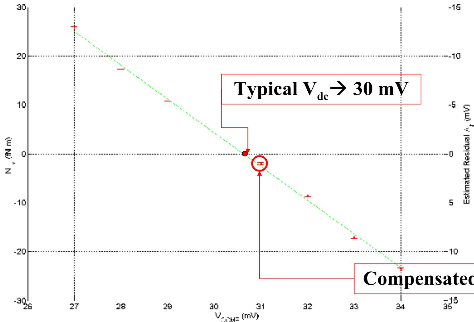
Compensation voltage on electrodes (mV)
