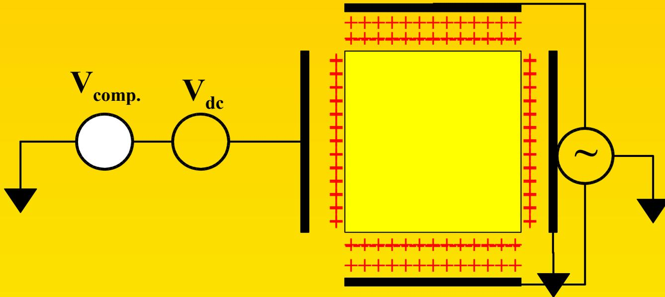
**Simulating a varying charge on the test-mass  $\rightarrow$  ac-torque induced**
