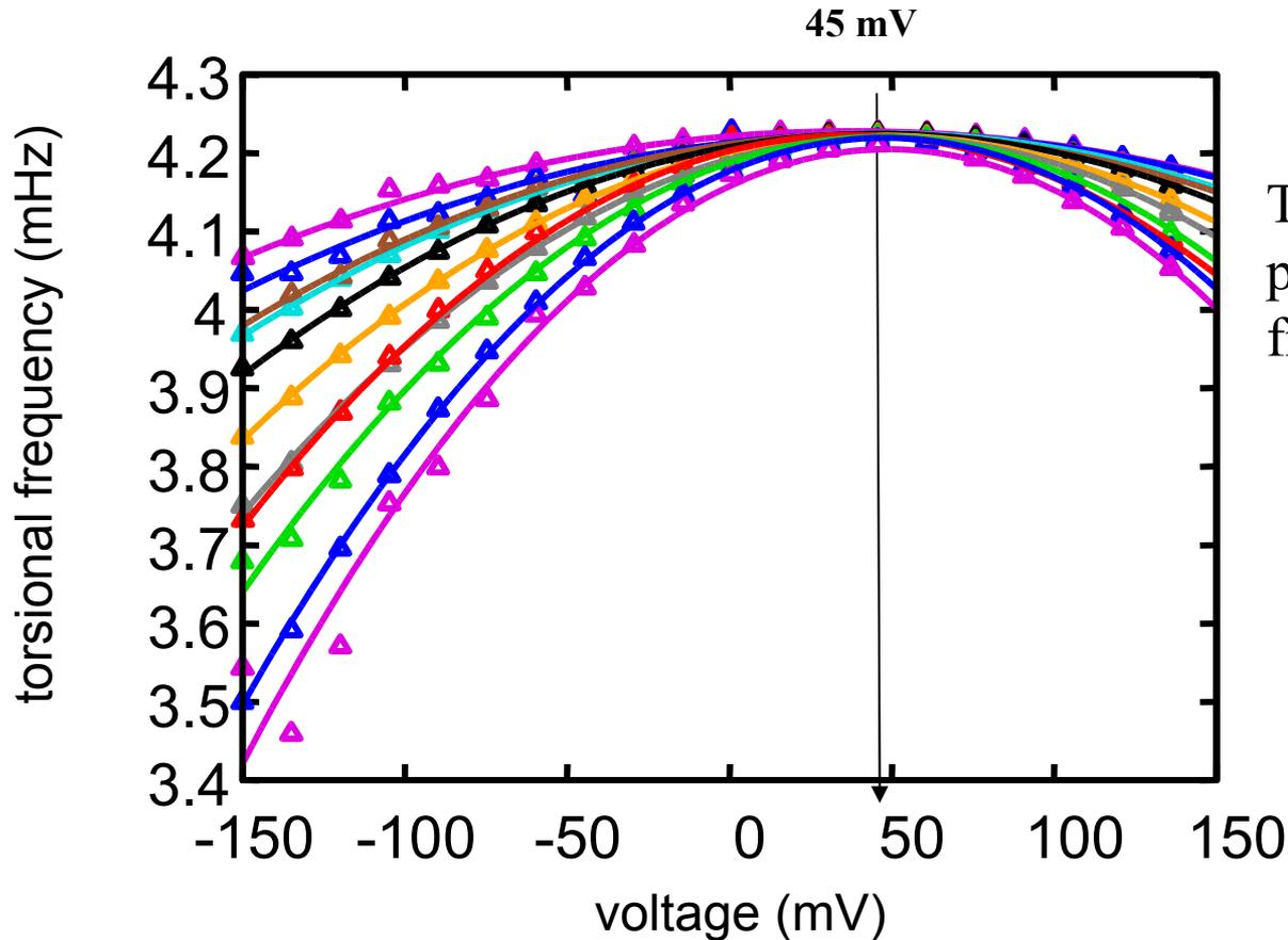
The different curves are for plate-pendulum separations,  $d$ , from  $d = 0.4$  mm to 0.75 mm
