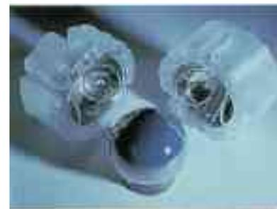
GP-B Flight Gyroscope
