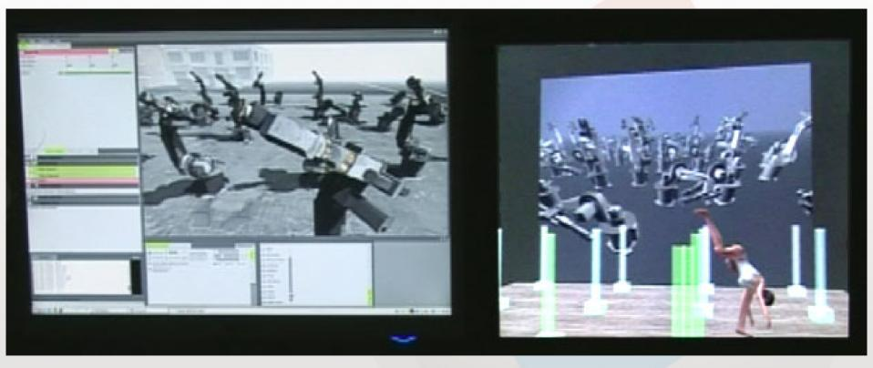
Performance Viewer: side-by-side comparison and validation of the transformation. From left to right: 3D visualization in Ogre3D, 3D model of the stage including the virtual dancer in VRML.
