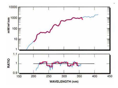
Comparison between SUSIM (NASA) and an earlier version of SOLSPEC on Spacelab 1 in 1983. A perfect spectrum is still the model the scientists are looking for.
