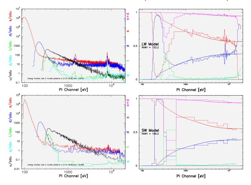
note the deficiency in Ni-K and Cu-K lines compared to FF/eFF mode because of the ventilation hole at the center
