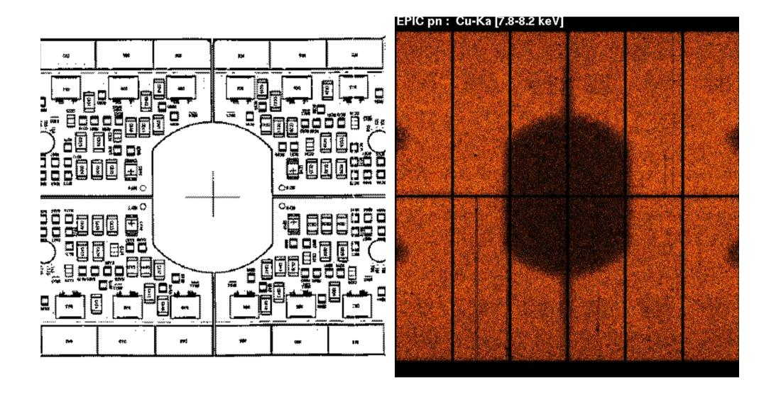
Printed circuit board: Cu + Mo (Ni + Au)
