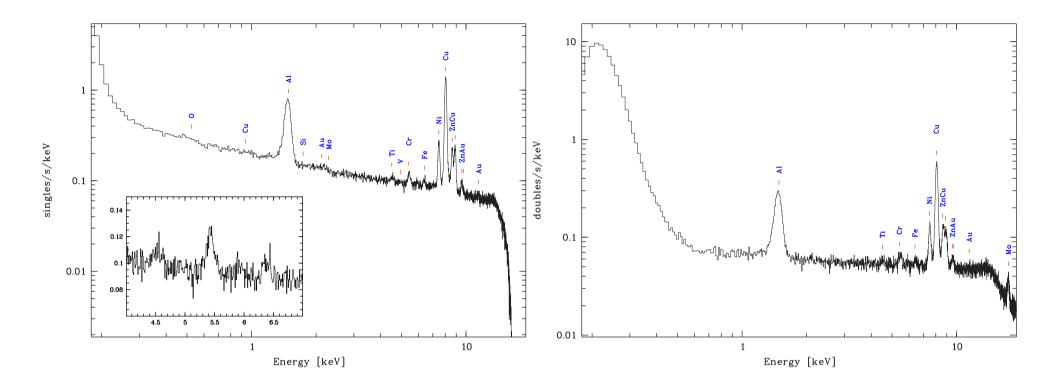
singles, doubles, 313 ks, FF mode Al-K, Ni-K, Cu-K, Zn-K, Mo-K Ti-K, Cr-K, Fe-K, Au-L Mo-K only in doubles, line position better than 0.3% background higher than in MOS (factor 2-4) could "easily" be reduced (factor  $\sim 5$ , graded shielding)
