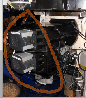
RINGO3 polarimeter with 3 cameras, fitted at the Cassegrain focus on the LT (credit: H. Jermak).
