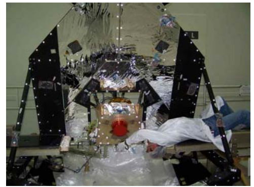
Two views of the integration of the Planck Cryo-Qualification Model spacecraft. At left, Alcatel technicians install part of the units in the Service Module (in particular, the HFI DPU can be seen with its massive harness). At right, the focal plane is being put in place. A cap placed over the HFI horns stands out in bright red.
