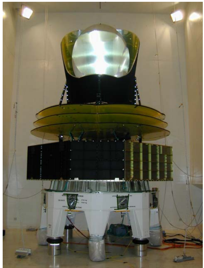
The Planck payload qualification model at Alcatel (Cannes), in the configuration used for acoustic testing. The qualification model of the primary reflector can be appreciated.
