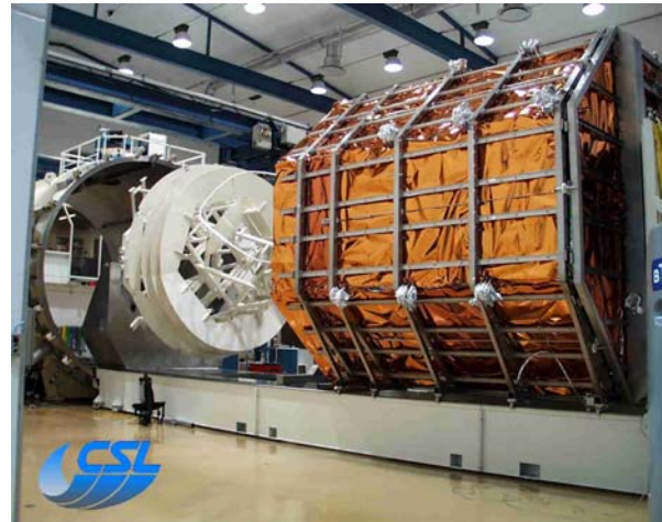
The actual facility at CSL, showing the vacuum tank, the mechanical mock-up used for the first test on the stand that will hold the satellite, and the helium-cooled shroud. The latter are on rails for insertion into the tank.
