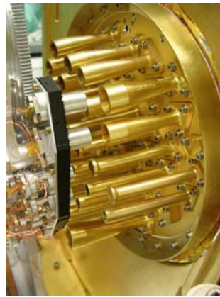
Cross-talk horns (left) in front of HFI horns, on the IAS Saturn calibration set-up
