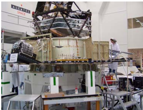
Two views of the integration of the Planck Cryo-Qualification Model spacecraft. At left, Alcatel technicians install part of the units in the Service Module (in particular, the HFI DPU can be seen with its massive harness). At right, the focal plane is being put in place. A cap placed over the HFI horns stands out in bright red.
