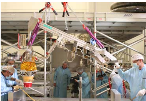
The handling of the HFI FPU integrated on dedicated equipment supporting the dilution cooler and 4K cooler pipes.
