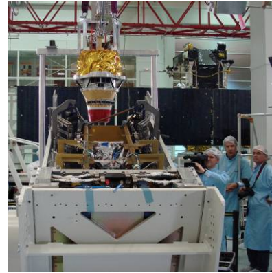
The HFI FM is carefully lowered into the LFI FM during one of the most critical phases of the instrument integration at Alcatel Cannes.
