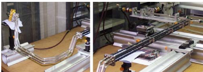
LFI QM waveguide assembly at 30 GHz under test at Istituto di Fisica dei Plasmi, CNR. Each assembly includes 4 waveguides connecting a front-end and a back-end module. Left: Copper section. Right: Stainless steel section.
