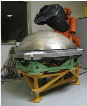
The mould for the secondary reflector.
