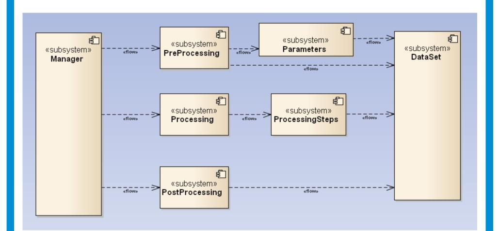
This simulator has been built under modularity principles in order to be generalized for the application to other space missions and other types of detectors. Each of the effects applied to generate a synthetic image are separated in a different module or "processing step".
