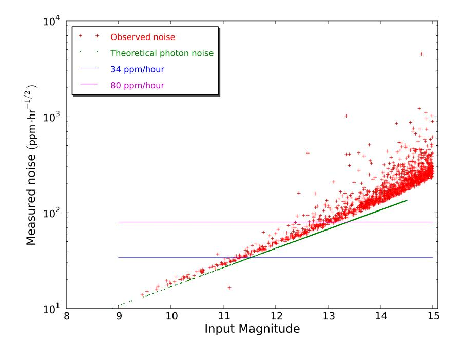
Noise-to-signal ratio as a function of the input magnitude. The deviation of the measured NSR from the theoretical photon noise occurs because only a fraction of the stellar flux is measured in the photometric algorithm. Two horizontal lines represent the noise limits at 34 and 80  $ppm\ hr^{-1/2}$  defined as mission requirement [2].
