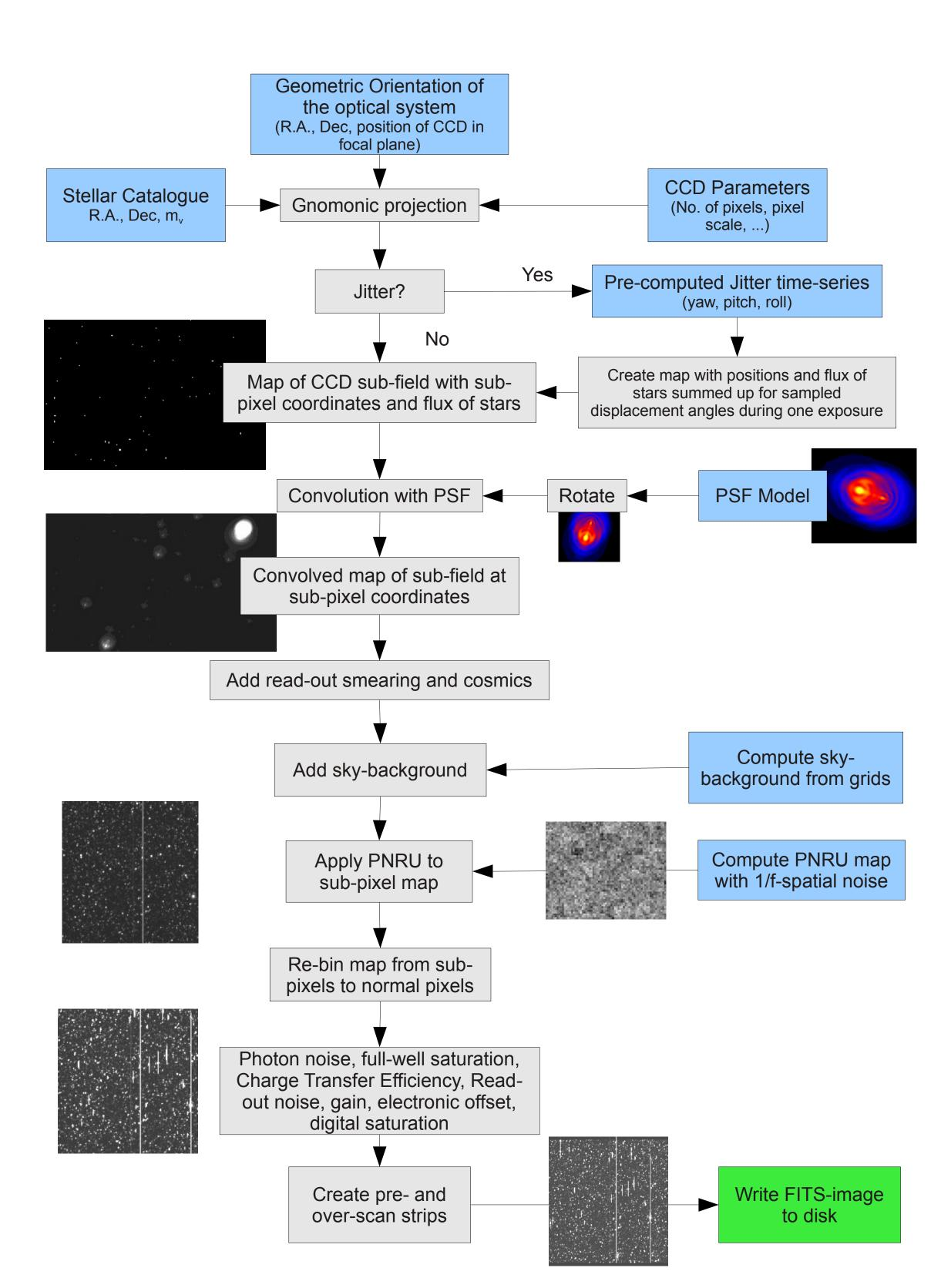
Several sources of noise for the instrument have been included and modelled. These include readout noise, readout smearing, full-well saturation, and digital These have saturation. modelled same way as described in [1].
