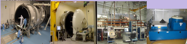
Thermal vacuum and other test facilities. Test equipments at ERIOs (Lab. d'Astrophysique Marseille) and SERMS (Univ. of Perugia).
