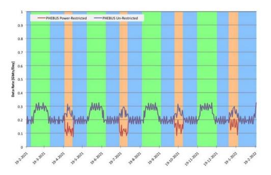
Data rate for PHEBUS for one terrestrial year – with and without restrictions.
